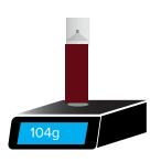
\*\*Secure the green silicone cap and the clear safety cap to each of the concentrating devices. Match the concentrating devices to +/- 1.0g of each other.
