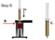
**A.** Place 60mL Syringe vertically on **XCELL** concentrating device
