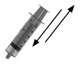
Prime the other syringes to ensure that the barrel moves freely. This is done by simply pulling back and forth on the plunger two to three times. Leave 5mL of air in syringe to prevent splatter
