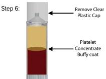
After spin, carefully remove **XCELL** concentrating devices from the centrifuge. Remove the caps from Step 4
