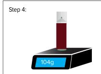
\*\*Secure the green silicone cap and the clear safety cap to each of the concentrating devices. Match the concentrating devices to +/- 1.0g of each other.
