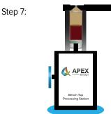
Insert **XCELL** Concentrating Device into Bench Top Processing Station then twist DIAL to move plasma to the bottom of the Luer-slip fitting.
