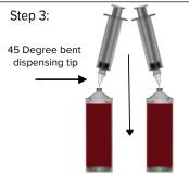
Slowly transfer anti-coagulated whole blood from each 60mL syringe using the 45 degree bent dispensing tips into two separate XCELL concentrating devices.
