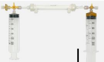
Step 12 Aspirate 4mL protein concentrate by drawing back the opposite syringe. Turn the stopcock to seal the port, remove and cap the syringe.
