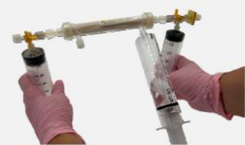
Step 9 Transfer plasma back and forth between syringes @5mL/1 sec rate until plasma is gone. Observe abundant water in the Vaclok.
