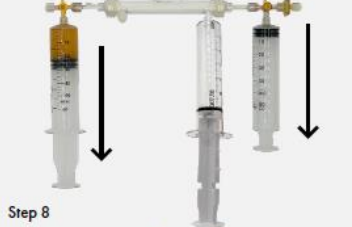
Step 8 Hold both 60mL syringe and tangentially process using a table or bench.
