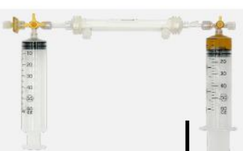
Step 12 Aspirate ~8mL protein concentrate by drawing back the opposite syringe. Turn the stopcock to seal the port, remove and cap the syringe.
