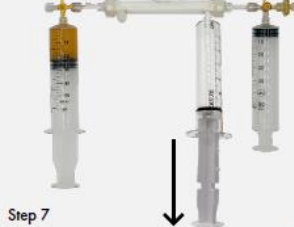
Step 7 Remove one of the white caps on the bottom of the filter, connect Vaclok syringe, and draw back to 60mL.
