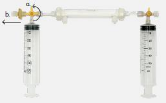
Step 11 a. Compress the air filter-side syringe, close the stopcock. b. Remove the air filter cap.
