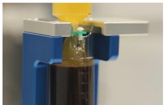
8. Detach the PPP Syringe and cap using the provided Luer Lock Universal Cap and set aside.
